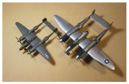
Scale models of Lockheed's P-38 "Lightning": and XP-58 "Chain Lightning" to show comparative sizes and designs. Both of these aeroplanes were considered to be obsolete and unnecessary after the end of WWII. tional front end cooling.
