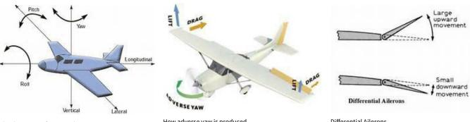
The three axes of an aeroplane.
