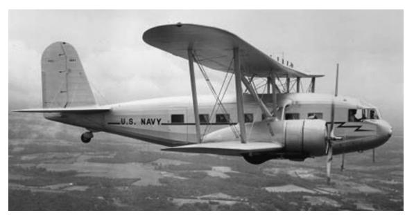
U. S. Navy R4C-1. military version of Curtiss "Condor". NACA cowlings, mostly retractable undercarriage, fairly streamlined fuselage and all of this with those old-fashioned strut and wire braced biplane wings. What's wrong with this picture? Note the familiar-looking Douglas DC-type fuselage profile.
