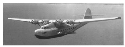
The streamlined and efficient early model Martin M-130 made the most of its total 3,800 hp whilst its competitors required 4,800 hp and more to perform the same task. Photo circa 1940
