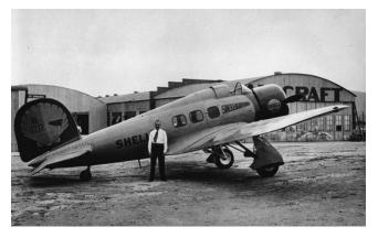
Vega, the 1928 Model 8 "Sirius," of which a special floatplane version was built for Charles Lindbergh, the 1930 "Altair," essentially a retractable-undercarriage variant of "Sirius" and one of the first aeroplanes so designed, and the 1931 Model 9 "Orion," a large and powerful six-passenger, retractable undercarriage airliner whose top airspeed of 220 mph at sea level was faster than U.S. military aircraft of its time.
