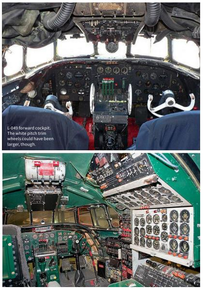
Got enough stuff? With the Co-Pilot's seat removed for clarity, the Flight Engineer's station on the right in the foreground and he Co-Pilot's switch panels on the right forward side of the cockpit are just a part of all that the crew of piston-engine airliners in the 1950's had to deal with. Jets are so much simpler. Note the plethora of engine controls under the main panel at the Flight Engineer's station.
