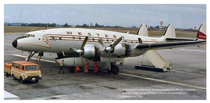
tric hoists. To facilitate moving it on the ground, recessed wheels were located under its front and back. Used mostly on shorter routes, Speedpaks were usually only carried when the weight of the passengers and fuel-on-board were low enough to permit the extra cargo load.
