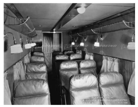
wide cabin (see photograph below); however, unlike the Fokker and Ford cantilever monoplanes, it was a biplane. This arrangement was selected to give the Model 80 a service ceiling sufficiently high so that unlike the Fokkers and Fords, it could fly over all but the highest Rocky Mountain ranges that lay along its route. This was before Federal Air Regulations prohibited flight with passengers above a cabin altitude of 8,000'.
