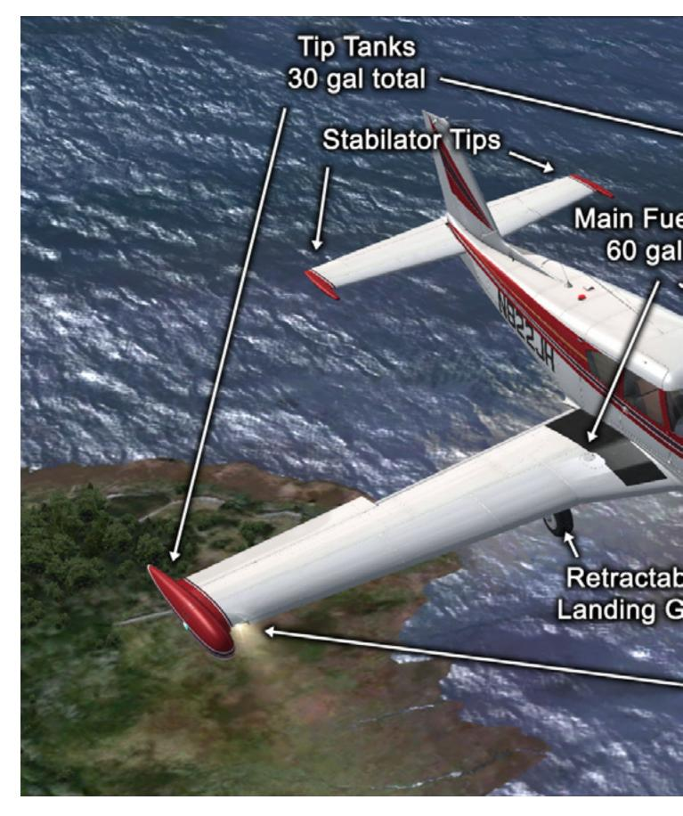
el Tanks total High strength, Wing Laminar Flow 250 hp Lycoming 540 6-cyl Engine
